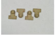
Fit the axle boxes to the wheel hubs ensuring that no glue gets into the wheel bearing.
