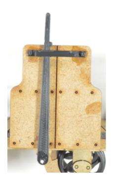
Glue the brake handle bracket to the seat end piece a couple of mm from the top then fit the brake handle behind the bracket and onto the rod ensuring the lugs on the brake handle are facing to the right. Trim off any excess rod flush with the break handle.
