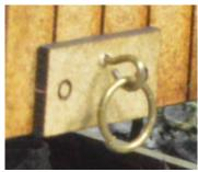
Locate the fret 1mm Parts #1 which is the back plates for the safety chains. Push the pin through the small hole in the plate ensuring that the engraved detail is facing out, trim off the pin to 3mm length and push the pin into the hole near to the bottom of the end piece and ensure that it is aligned with the bottom edge.
